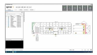
As in all systems, devices in the monitoring and control of card access systems are divided into two as input and output devices due to their duties. The list of devices in the system can be accessed via the "Card Pass" easy indicator in the upper right corner. The devices in the system can also be displayed on the map in the same way.
